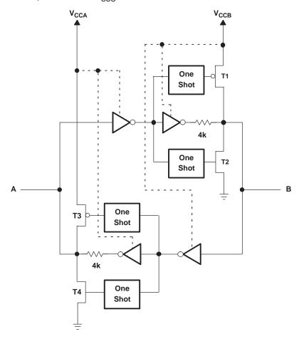
Figure 1. Architecture of TXB0101 I/O Cell
